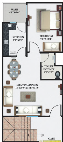
DUPLEX FLOOR PLAN PLOT SIZE - 16'0" X 35'0" PLOT AREA - 560.00 SQ.FT.
